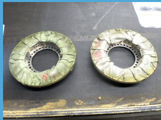
After spraying: DeWAL Plasma X tape on front/back of part
