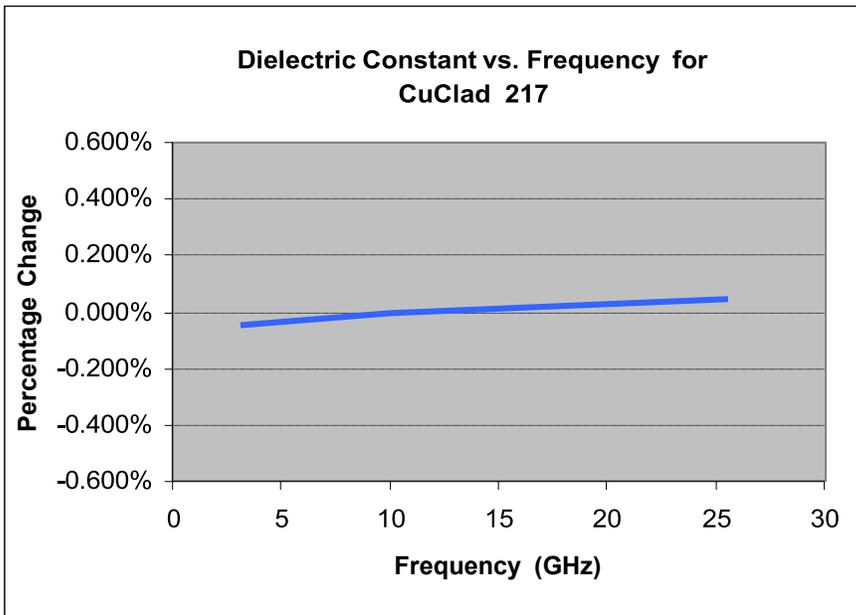
Demonstrates the stability of Dielectric Constant across Frequency. This information was correlated from data generated by using a free space and circular resonator cavity. This characteristic demonstrates the inherent robustness of Rogers' laminates across frequency, thus simplifying the final design process when working across EM spectrum. The stability of the Dielectric Constant of CuClad 217 laminate over frequency insures easy design transition and scalability of design.
