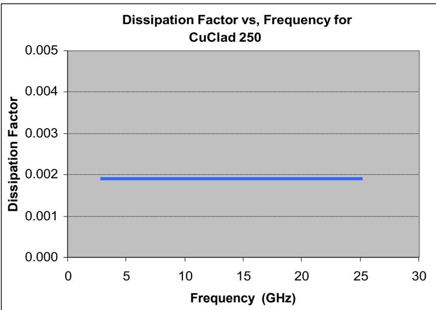
Demonstrates the stability of Dissipation Factor across frequency. This characteristic demonstrates the inherent robustness of Rogers' laminates across frequency, providing a stable platform for high frequency applications where signal integrity is critical to the overall performance of the application.
