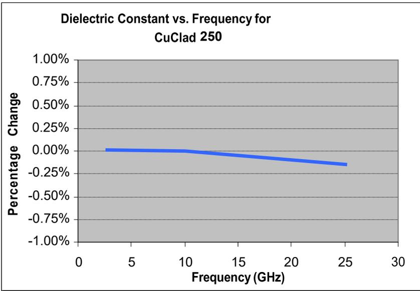
Demonstrates the stability of Dielectric Constant across frequency. This information was correlated from data generated by using a free space and circular resonator cavity. This characteristic demonstrates the inherent robustness of Rogers' laminates across frequency, thus simplifying the final design process when working across EM spectrum. The stability of the Dielectric Constant of CuClad 250 laminate over frequency insures easy design transition and scalability of design.
