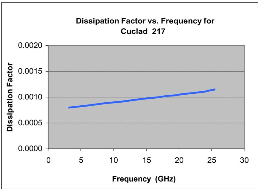
Demonstrates the Stability of DissipationFactor across Frequency. This characteristic demonstrates the inherent robustness of Rogers' laminates across frequency, providing a stable platform for high frequency applications where signal integrity is critical to the overall performance of the application.
