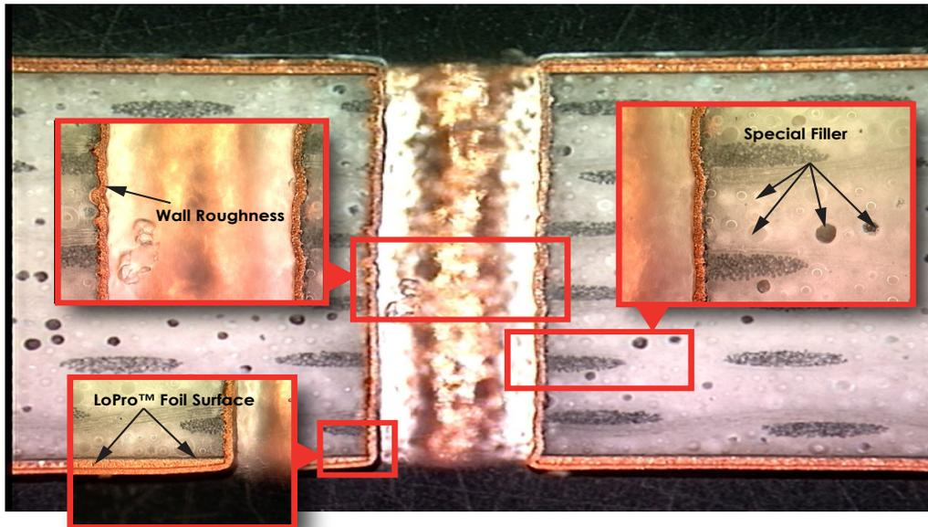
Figure 1: Cross-section of a typical RO4730G3 laminate plated through-hole. Note that the appearances of the special filler and slightly increased hole-wall roughness are normal for this product. Additionally, the LoPro foil surface contains a thin coating of modified base resin, which appears colorless. We suggest discussing hole quality/appearance with a Rogers' Technical Service Engineer prior to processing RO4730G3 laminates for the first time.
