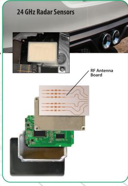
Rogers' RO4835<sup>™</sup> laminates provide the superior electrical performance and consistency needed for reliable automotive radar antennas at 24 GHz. With 10X improved oxidation resistance compared to traditional thermoset materials, RO4835 laminates feature stable low-loss performance over time.
