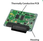
ML Series<sup>™</sup> laminates and prepregs are thermally enhanced to conduct and spread heat and eliminate hot spots. Capable of single and multilayer constructions, these materials are used in parts where power IC thermal management is an issue, such as power converters, power supplies and ECUs.
