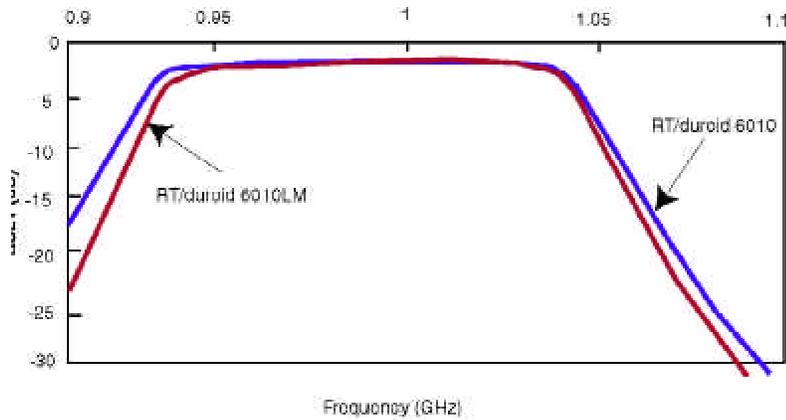
Graph 1. Initial S<sub>21</sub> response of Band Pass Filter (RT/duroid 6010LM inside curve)
