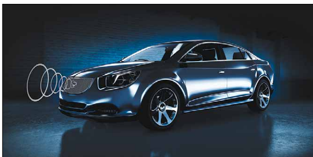
▲ Fig.1 Radar mounted behind the front emblem, which is a radome.
