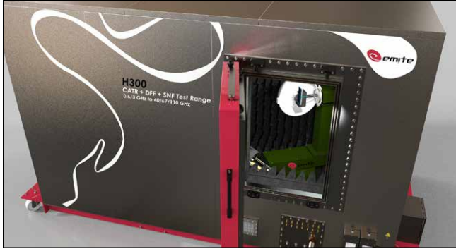
▲ Fig. 6 EMITE H-Series 600 MHz to 110 GHz small anechoic chamber including climatic enclosure.
