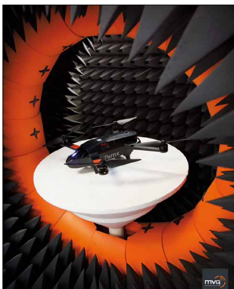
▲ Fig. 9 MVG's multi-probe system testing a drone.
