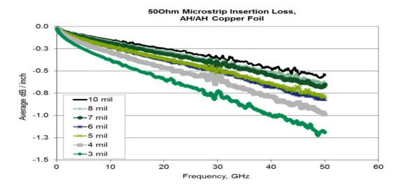
Figure 3. 50 Ohm Microstrip Insertion Loss
