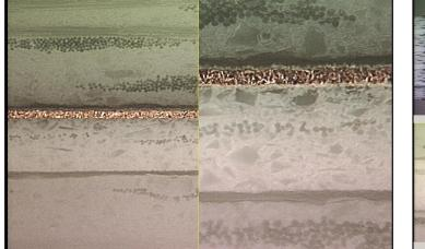
Expected visual appearance in a cross section of RO4000 LoPro laminates.
