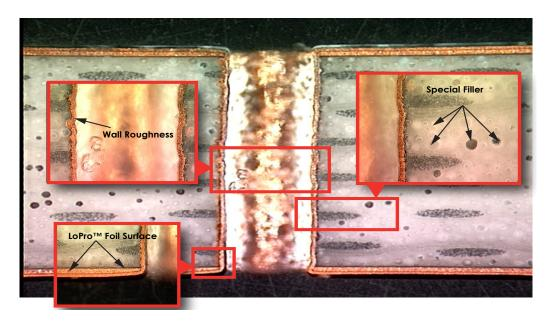
Figure 1: Cross-section of a typical RO4730G3 laminate plated through-hole. Note that the appearances of the special filler and slightly increased holewall roughness are normal for this product. Additionally, the LoPro foil surface contains a thin coating of modifed base resin, which appears colorless. We suggest discussing hole quality/appearance with a Rogers' Technical Service Engineer prior to processing RO4730G3 laminates for the first time.
