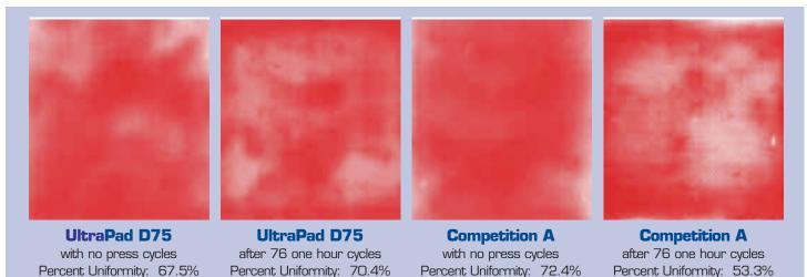
By utilizing imaging software, you can see that after 76 hours the fiberglass pattern is visible on pressure sensitive paper and the competitive product's service life has ended. After 76 hours, UltraPad has simply conformed to the press assembly yielding similar pressure uniformity as it had at the beginning of the test.
