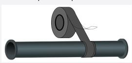
Continue elongating the tape and wrapping with half-laps until the object is covered to the desired extent.
