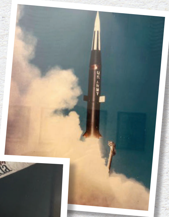
Above: Radome for Pershing II missile uses RT/duroid® to permit microwave transmission and to provide resistance to ablation, rain erosion and handling damage.
