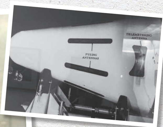
Left: On the Apollo moon landing program and the Space Shuttle, RT/duroid® PTFE composites did critical jobs in self-lubricating bearing parts and in microwave circuitry and antennas where stability in temperature extremes and radiation was essential.
